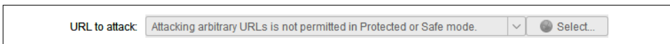
Figure 3-8. The URL to attack text box is grayed out due to the ZAP mode
