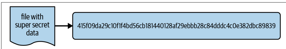
Figure 3-2. A file checksum is a unique value based on the contents of the file
